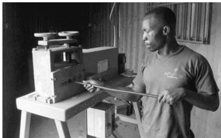
In this Nov. 26, 2018, photo, a man uses a wire-stripping machine to get to the copper and other metals in discarded electronic cables in Accra, Ghana.
